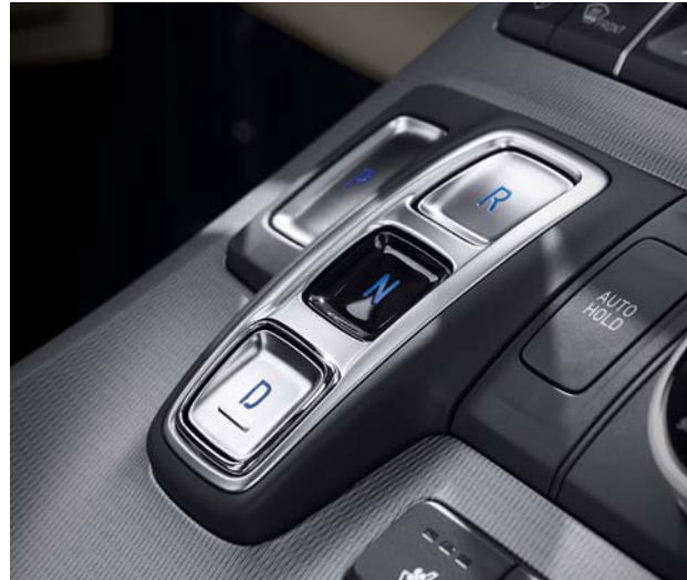
8-speed shift-by-wire automatic transmission
